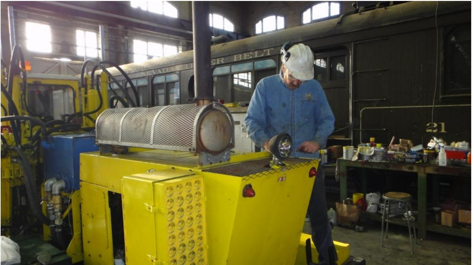
Fred fits the first segment of the leaf-guard/light-shield on the tie-shear.
