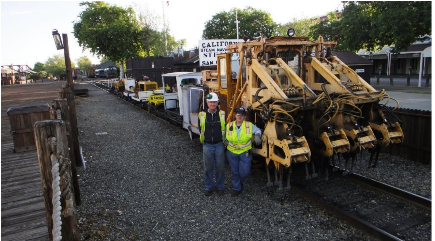
It's 8 o'clock a.m. and Steve N. and Heather have been on the job for two hours already assembling the MOW work-train. They're just waiting for the Kalamazoo tug pulling two flat-cars carrying ties and the bench-car to come over from the Shops. Shown here are the old-old tamper pulling the A-5 motorcar, rail-lifter, rail-mounted compressor, materials car, tool car, spike puller, and A-6 motorcar. The Jackson 125 tie-exchanger and scarifier-inserters are spotted just out of the picture by the L Street crossing.
