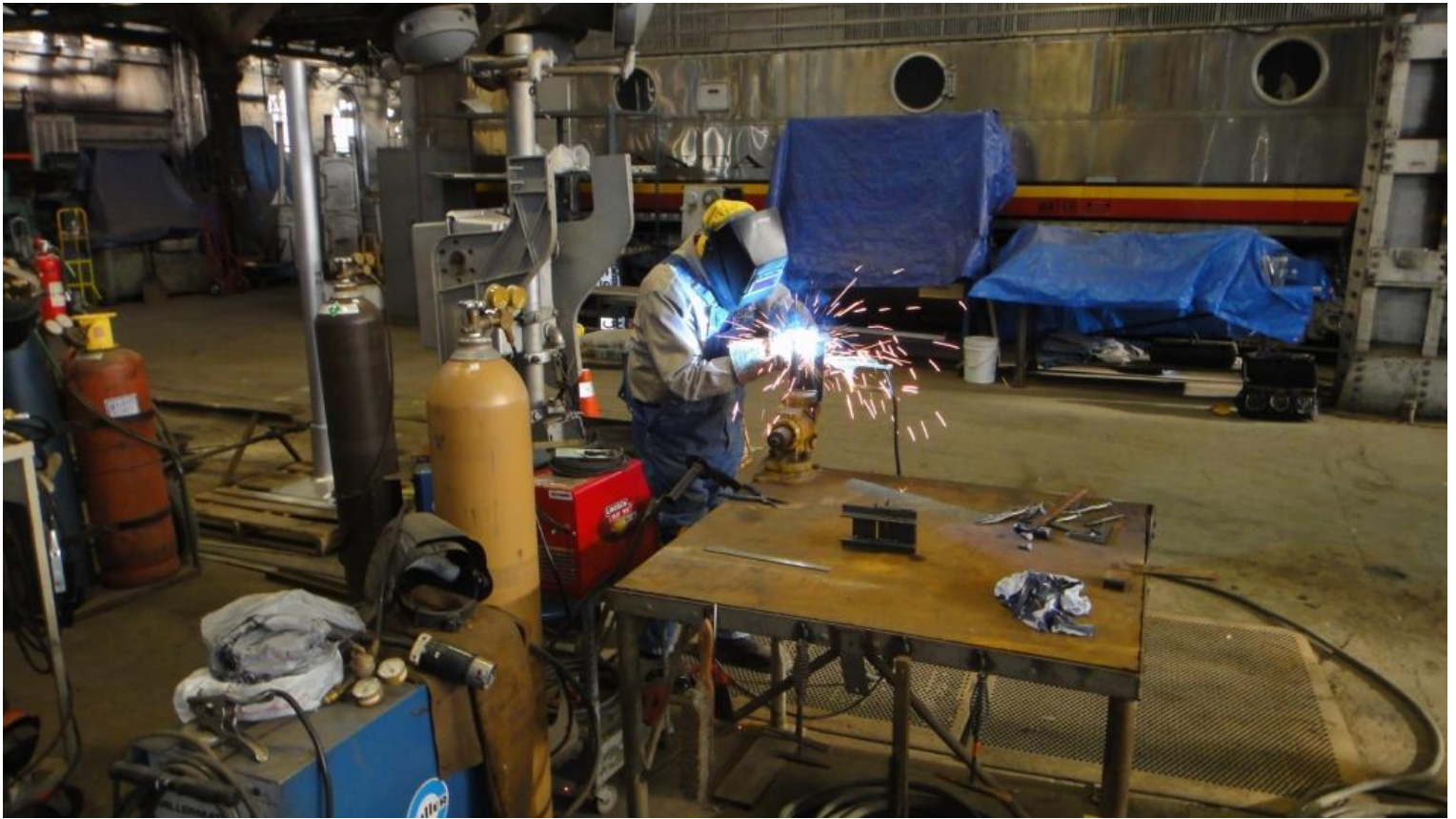
Cliff is a master of metal manipulation. Here he creates custom crafted brackets for the new leaf-guard on the tie-shear
